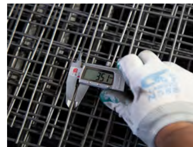
7 Mesh panel wire diameter test
