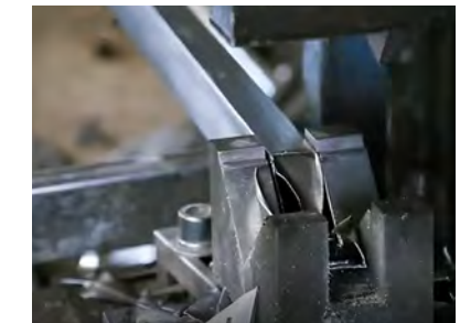
4 Square Pipe Cutting
