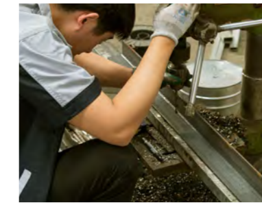
3 Angle Steel Punching
